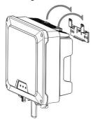
3. Check both sides of the heat sink to ensure that it is securely in place.
