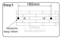
After drilling holes in the wall, place two screw anchors into the holes, then attach the wall mounting bracket to the wall using the self-tapping screws and washers delivered with the inverter.
